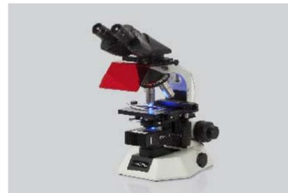
1. The LED based transmitted fluorescence attachment uses a unique proprietary illumination system, allowing significant increase in performance and cost reduction. The microled comes with a choice of blue, royal blue and green LED cassettes.
