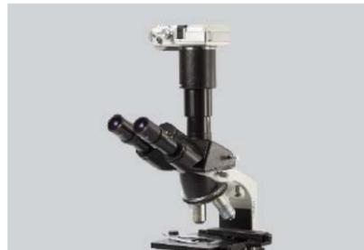
2. The Trinocular Head comes with a wide range of camera adapters that allow users to mount various kinds of digital cameras onto the trinocular head of the microscope for quick and easy digital documentation.
